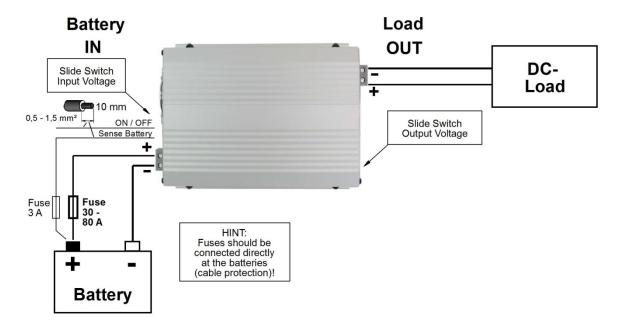
First connect the DC-DC converter, after that the battery.
